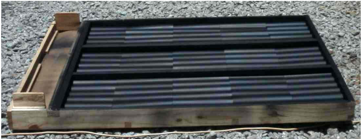
Fig. 71: Coated air collector before mounting the glass cover.
