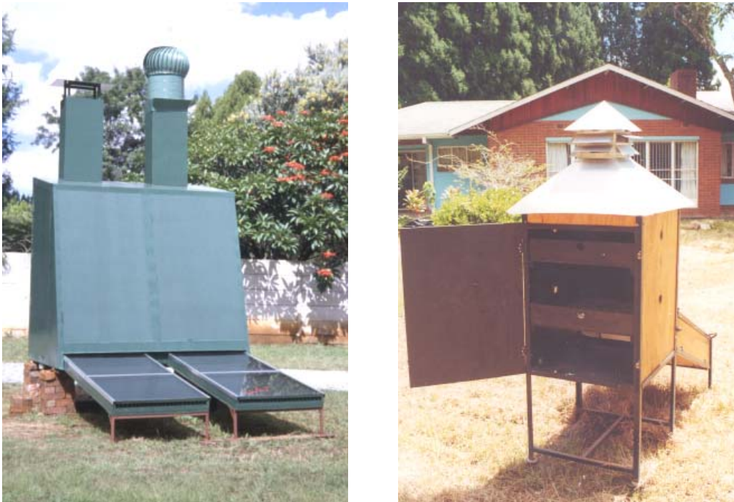
Fig. 16: Passive cabinet solar dryers in Zimbabwe (Domestic Solar Heating left, DTC, UZ, right)
