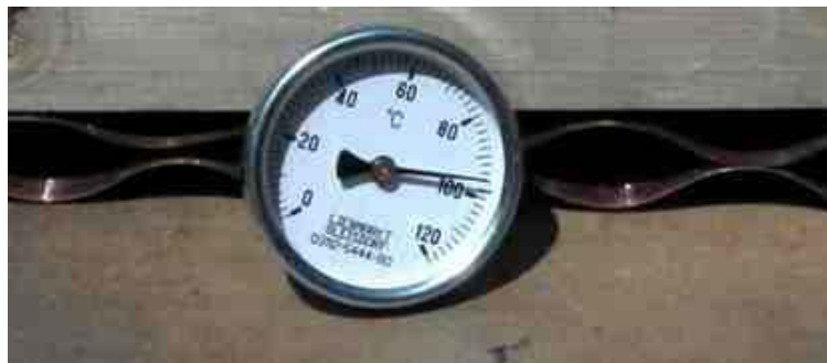
Fig. 72: Measuring the air temperature inside the collector.
