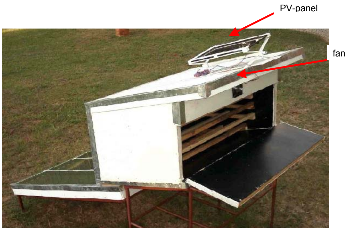
Fig. 21: The fan is powered by a 6 W PV-panel.
