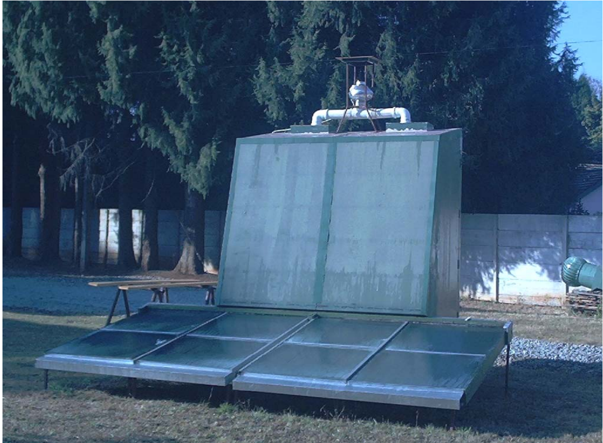
Fig. 18: Active ventilated cabinet dryer with fan on the top (Harare, Zimbabwe)
