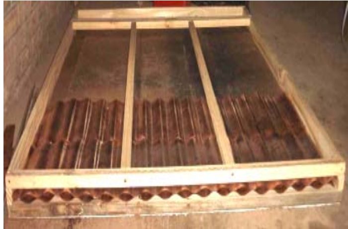
Fig. 70: Prototype of the air collector prior to the coating with black paint and without glass cover
