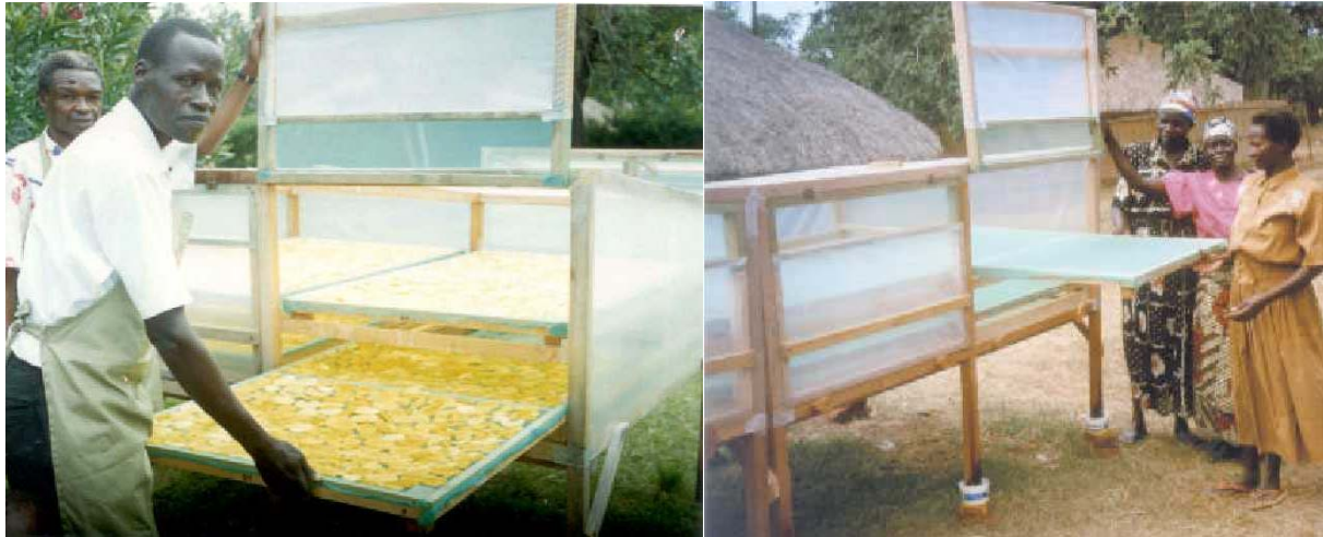
Fig. 42: Pictures of the Mango solar dryers in Uganda (passive direct solar cabinet dryer) [5]
