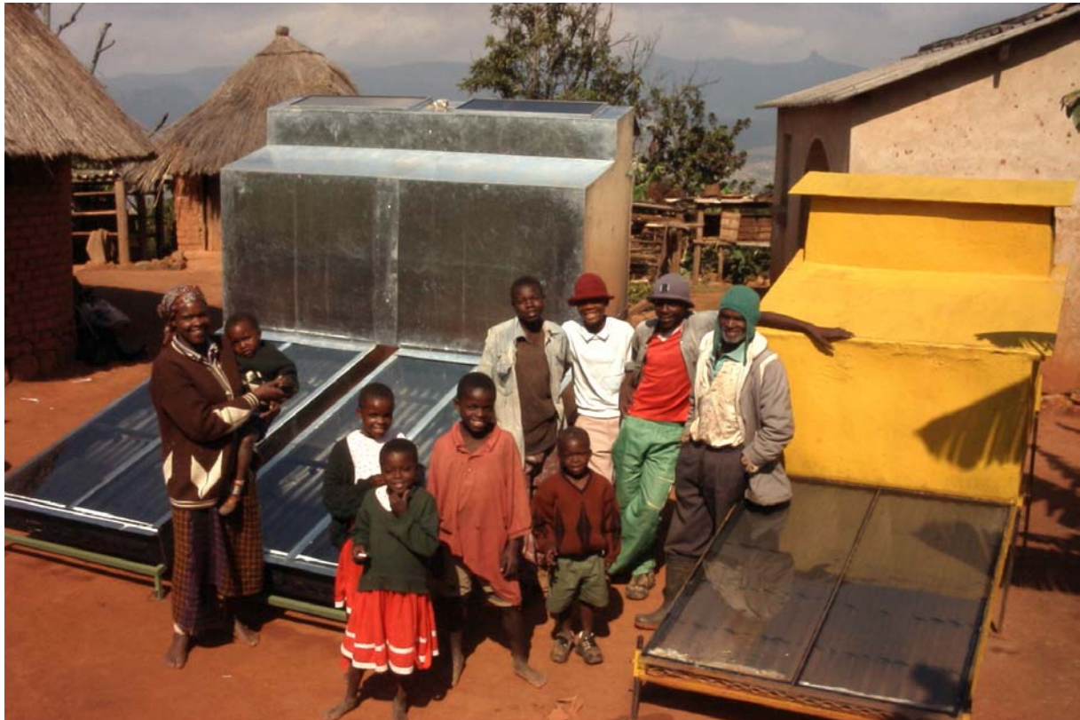
Fig. 49: PV-powered forced convection solar coffee dryer (left) and natural convection cabinet solar coffee dryer (right) at a farmers co-operative in the Honde valley, Zimbabwe
